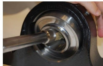
Figure 4 — Torquing bearing 90° into housing
