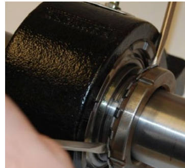
Figure 2 — Zero Shaft Fit: Pry against housing to draw adapter sleeve through bearing. Sleeve should not be protruding out the backside of the inner ring.
