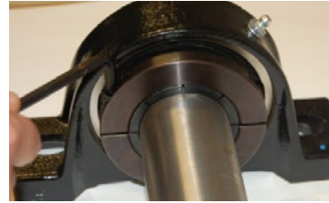
Figure 2 — Zero Shaft Fit: Pry against housing to draw adapter sleeve through bearing. Sleeve should not be protruding out the backside of the inner ring.
